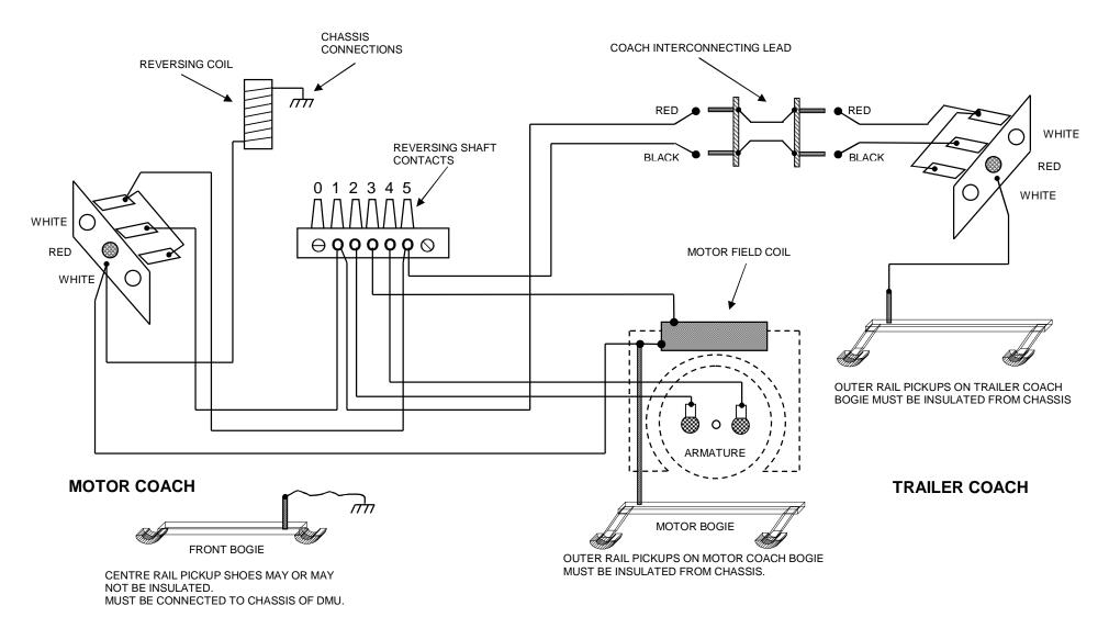
IF RED LAMP AT FRONT END LIGHTS WHEN MOTOR COACH RUNS FORWARDS, CHANGE WIRES 2 AND 4.
