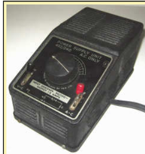
The TTR AC Power Unit 492 incorporates the same controller mechanism and safety cut out. The knob is not interchangeable with that of the Controller type 472.
